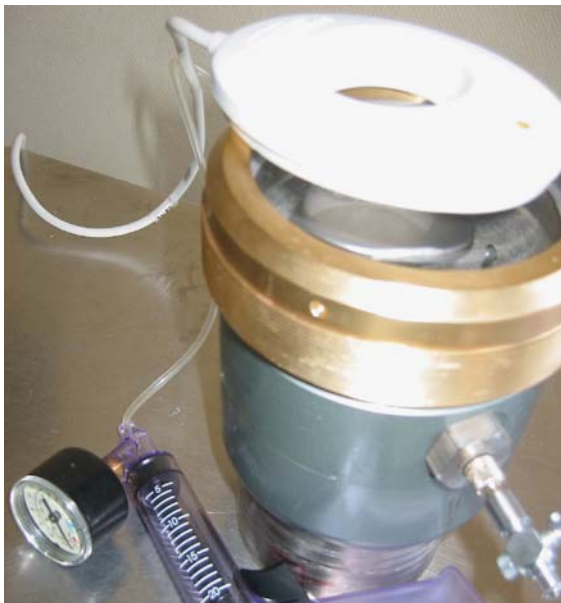
Fig. 1 The pacemaker was placed in the hyperbaric chamber, and the inflation system was connected to the chamber with the telemetry wand positioned on the cover
