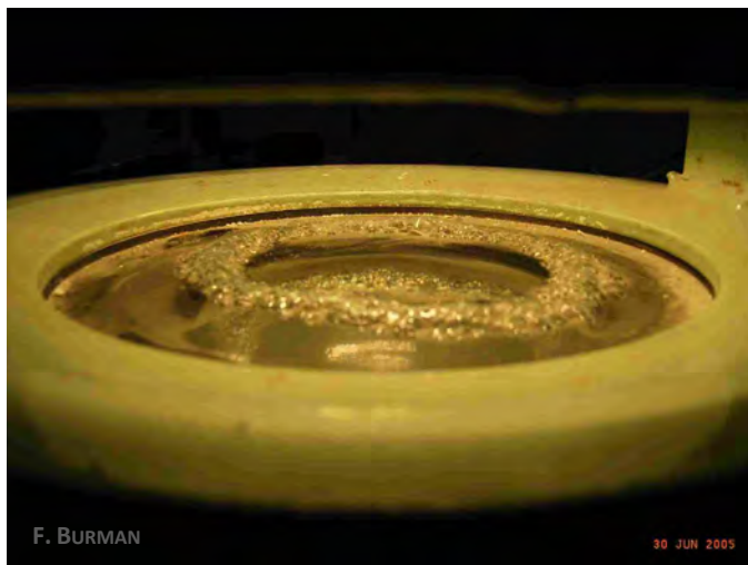
Acrylic and heat don't mix. Be careful of the lamp you use!
