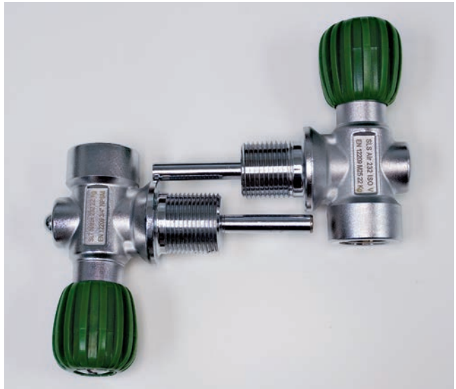
The valve on the left is suitable for 3/4-inch NPSM cylinder threads. The valve on the right will erroneously thread into a 3/4-inch NPSM cylinder neck for about three to five threads before it begins to bind.
