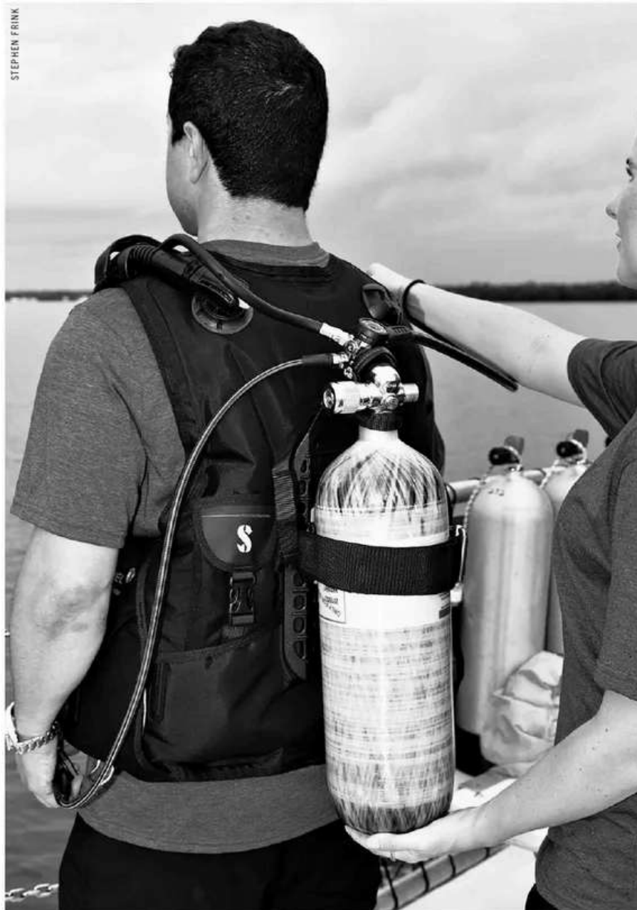
Some Type 3 (aluminum-lined) cylinders are allowed for use in water, but Type 4 (polymer-lined) cylinders are much more suitable for scuba. If either of these composite cylinders are to be used in water, there are many pros and cons to consider.
